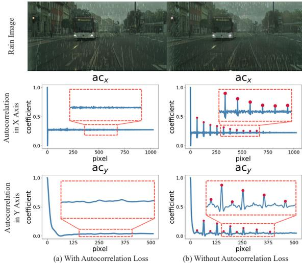
Figure 5. Comparison of results w/o autocorrelation loss. The rain image and corresponding autocorrelation along x and y direction are compared between the result (a) with autocorrelation loss, and (b) without autocorrelation loss (peaks marked with red points).
